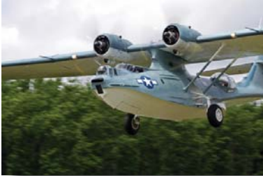
The PBY Catalina does everything leisurely, albeit impressively. Retracting the landing gear is one of those. Here the Catalina is shown soon after lift off with the nose gear retracted before the mains begin to fold up.
