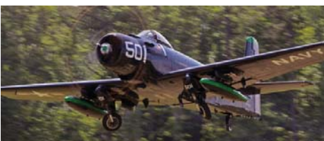
Both the main gear on the Douglas AD "Able Dog" Skyraider retract simultaneously, but twist 90 degrees to sit flat inside the wing.
